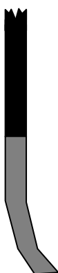
Figure 19: Open face can be achieved by bending the lower part of the blade forward.
