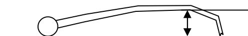
Figure 17: The hook is measured between the floor and the highest point of the lower end of the blade.
